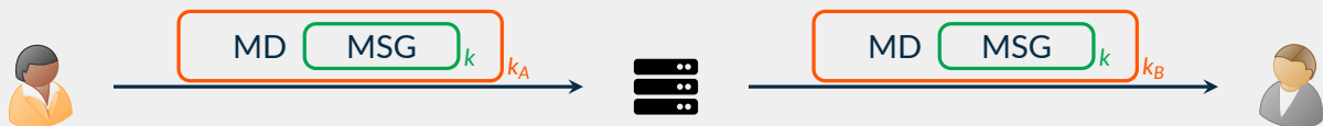
Figure 3: Transport encryption and end-to-end encryption (E2EE). \boxed{\text{DATA}}_k indicates that DATA is encrypted using the symmetric key k . We use distinct colors for end-to-end encryption and transport encryption. The server shares a transport encryption key k_A with Alice, another key k_B with Bob, and can therefore read the metadata MD. However, the end-to-end encryption key k is only known to Alice and Bob, hence the server cannot read the message MSG.
